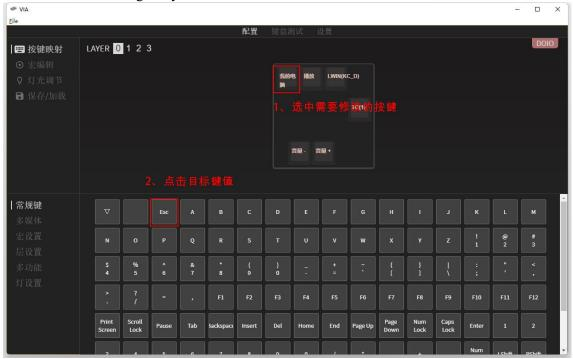
Players can define the keys of "layer 1" "layer 2" and others blank in VIA as your needs. After defining it, on the keyboard can get the new customize key by changing "TO" key to "layer 1" and "layer 2"
