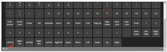
Other key value codes can be found by clicking the relevant key value in VIA with the mouse. There will be a code hint in the lower-left corner or you can view the relevant codes through this link:
