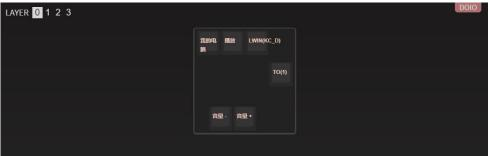
The second layer (" 1 "displayed on the VIA interface) is the PS function key value area, and the layout is defined as the common shortcut keys of PS
