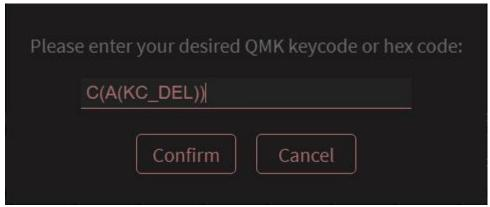
The figure above shows the combination key "CTRL+ALT+DEL". The "C" in the figure corresponds to the code of the ANY key for CTRL, "A" corresponds to the code of the ANY key, and "KC\_DEL" corresponds to the code for the delete key. Each individual key value is separated by a parenthesis, distinguishing each key. The end of the key value input should have an equal number of right parentheses.
