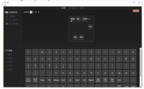
The first layer (" 0 "is displayed on the VIA interface) is the default key area, and the layout is the common multimedia key area.
