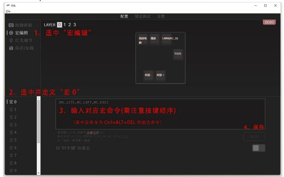
After changing the key value to the macro key in KeyMapping-Macro Settings, the corresponding key is a combination of CTRL+ALT+DEL when you press it.
