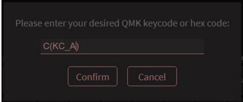
The figure above shows the combination key "CTRL+A". The "C" in the figure corresponds to the code of the ANY key for CTRL, and "KC\_A" corresponds to the code of the ANY key. Also, because there are only two keys, there is only one parenthesis to differentiate them. Now let's take a look at the ANY key code corresponding to each function key on the keyboard:
